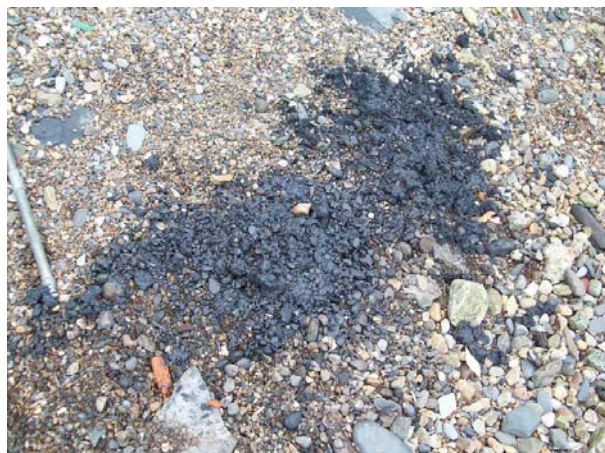
Photo E.12 – View of ground material from auguring for groundwater. Note: This material was rock and wet, greasy black material which had an odor of old fuel/oil. This material after being exposed to the air would gradually harden.
