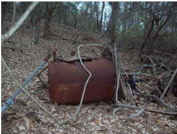
Photo E.21 – View of rusted out oil tank (empty) located within the area of the former water tower.
