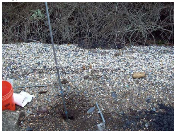
Photo E.11 – View of the proposed groundwater sample location. Note: After four attempts at auguring different locations, the groundwater sample was abandoned due to refusal from metal debris and cobble. The subsurface soil sample (GI-DA-SB-04-01) was collected in this location.
